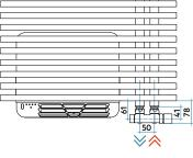
Type with collectors on the right Hydraulic connection 50 mm
